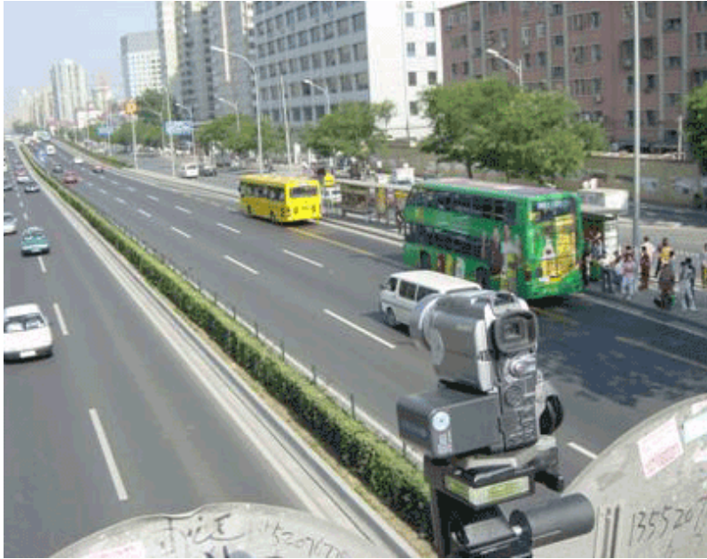
FIGURE 2a Collecting Vehicle Class Information using Video Cameras
